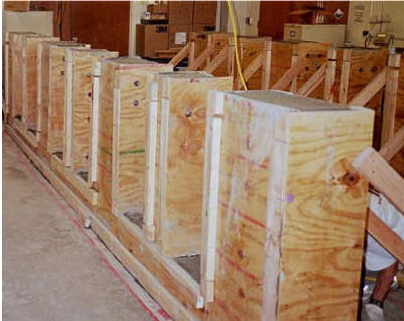
Figure 3.20 Test specimens shortly after concrete placement
