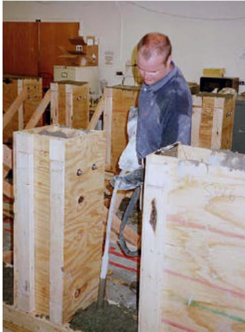
Figure 3.19 Internal vibration of SFRC
