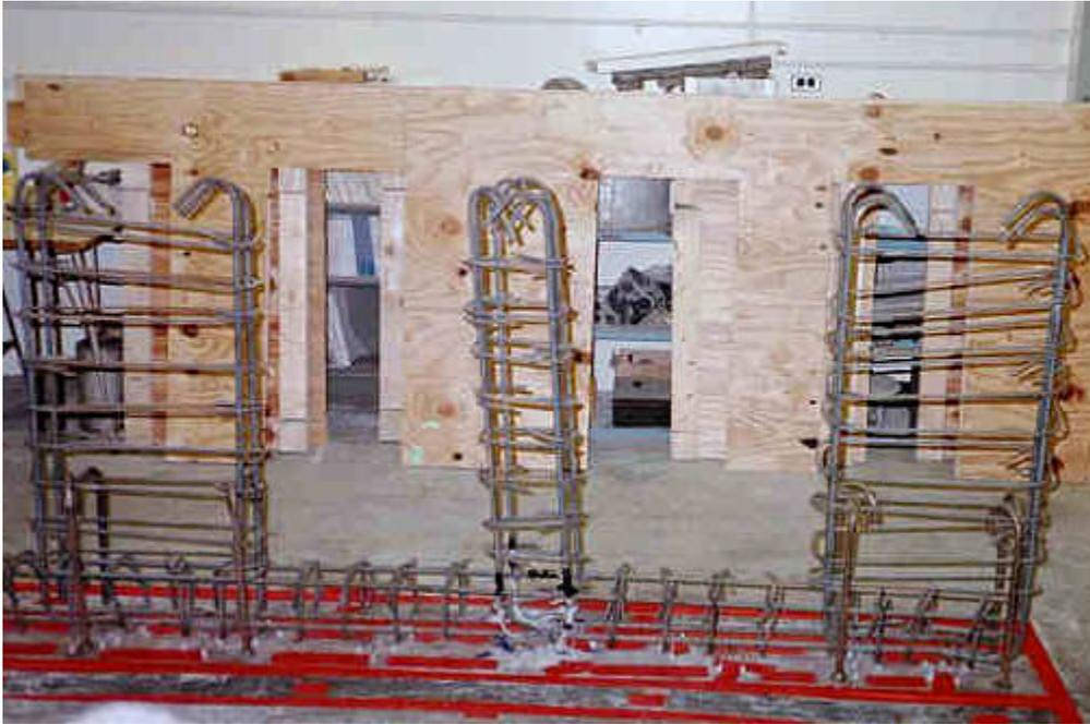
Figure 3.10 Bar arrangement under construction for a plain concrete test specimen
