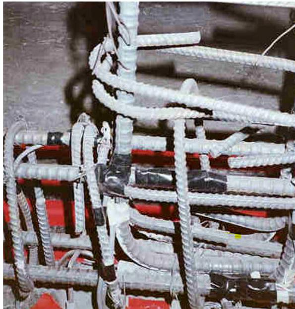
Figure 3.22 Protected strain gages
